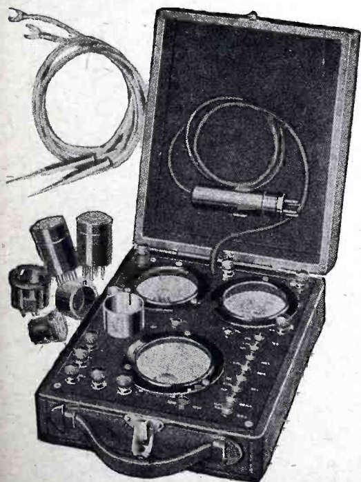
A radio test set used to check circuits, test tubes, "A" and "B" eliminators, batteries, voltages in circuits, etc., etc.
