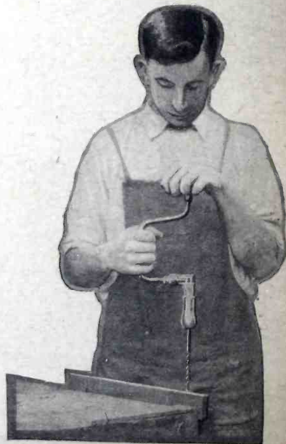
Boring for the dowels in a stile.
